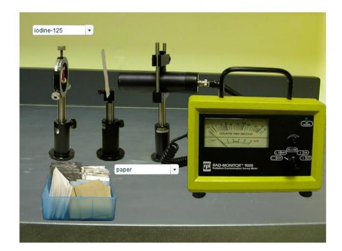
The gauge indicated radiation levels in "Counts per second". The nuclides used in this section are:
